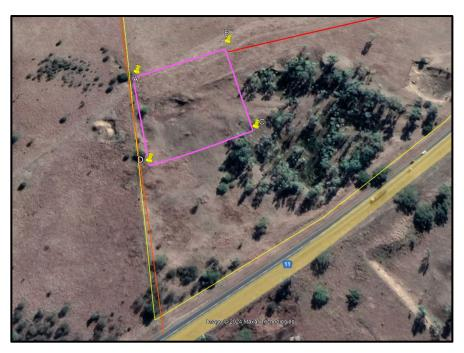
Figure 4: All mining will be >10 m from the adjacent power lines (orange line) (image obtained from Google Earth).
